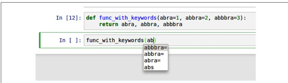
Figure 2-4. Autocomplete function keywords in a Jupyter notebook
